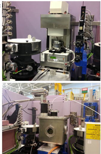
On the KOOKABURRA instrument sample environment equipment can be placed between the perfect Si crystal monochromator and analyser stages. Top: A rheometer for shear cell experiments. Bottom: A high-field magnet with cryostat temperature control.
