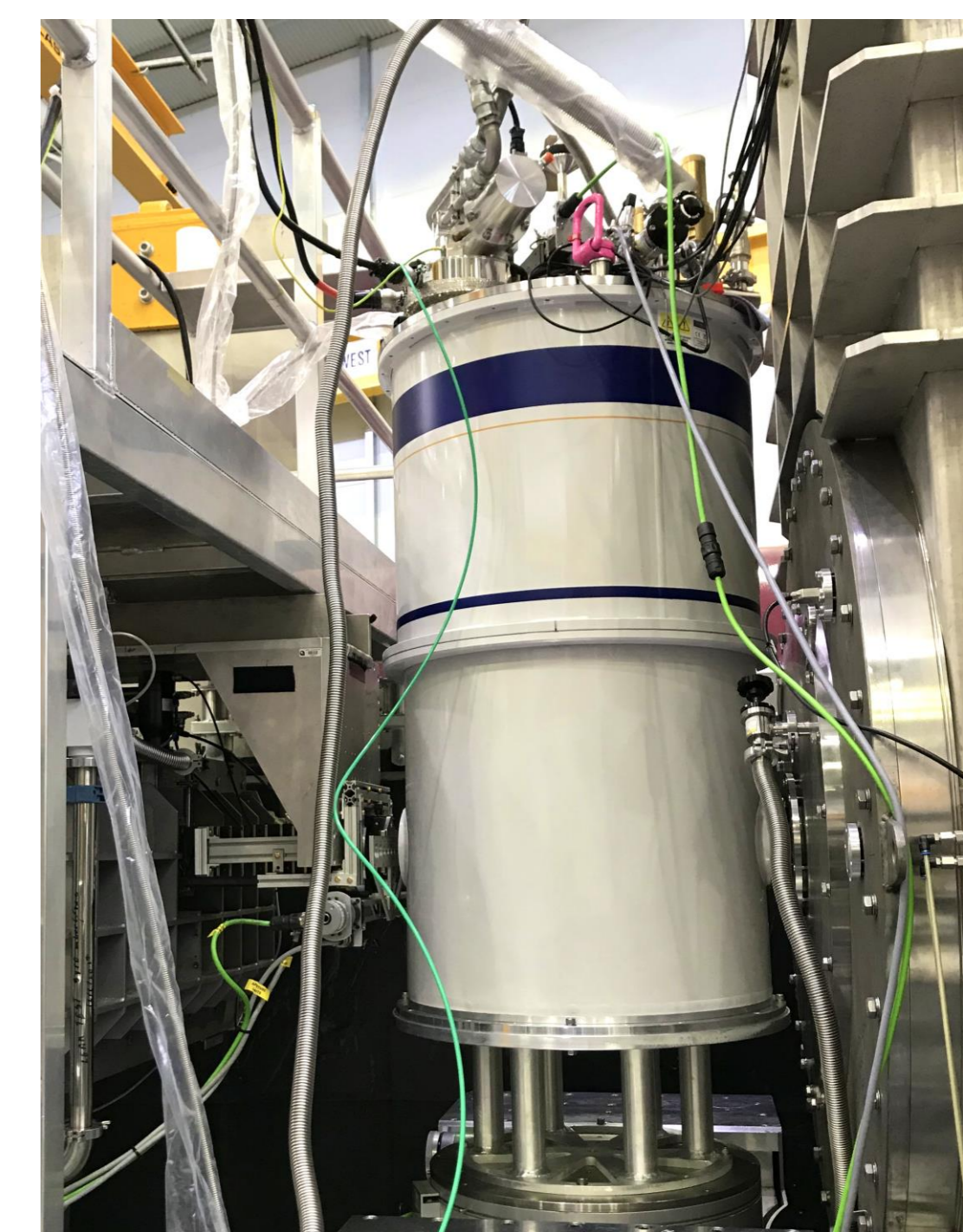
7 T compensated vertical magnet installed on Quokka
