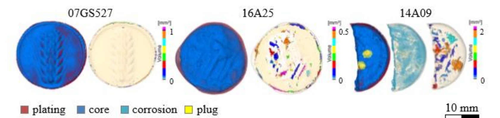
Figure 2: Left, the structural components are separated and rendered in different colour for each sample; the colour code is expressed by the legend on the bottom. Right, the maps show the distribution of porosities. A scale bar on the right side of each figure indicates the coding colour-volume.
