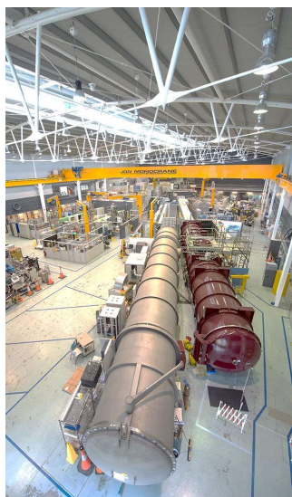
Figure 1. Photo of the neutron guidehall at ANSTO. QUOKKA is the SANS instrument on the left, adjacent to the BILBY the time-of-flight SANS instrument on the right of the photo.
